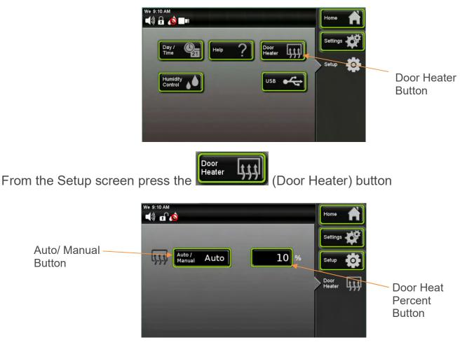
In Automatic mode, the door heater works in conjunction with the internal heaters to maintain the temperature set point. In the event that the temperature is above set point, the door heater will automatically throttle back.
