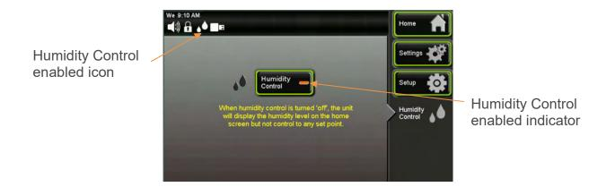
When the humidity control is enabled the toggle button indicator is on and the humidity control icon in the status bar has the red circle removed. Once the selection has been made the status of the Humidity control will be visible on the home screen.
