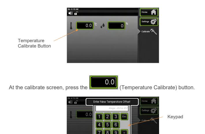
Enter the temperature offset by using the keypad and pressing complete.
