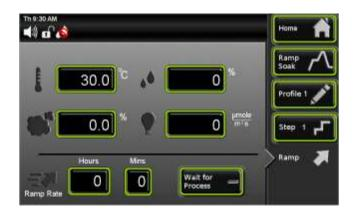
Ramp rate allows a user to control the rate which parameters (temperature, humidity, CO<sub>2</sub>, lights) change when transitioning to a new setpoint. This allows for a more gradual change than otherwise would occur. Temperature tolerance range is 1°C when ramping temperature. Humidity tolerance is 2% when ramping humidity.
