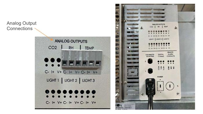
Analog outputs provide either a milliamp (4-20mA) or voltage (0-5V) signal output to represent each of the displayed temperature (and humidity) values. These options can be used for connection to in-house data acquisition, recorder, or alarm system. The temperature parameter (only) is adjustable in its scaling and is accessible at the Analog Output screen.
