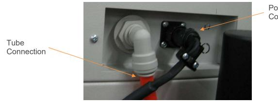
Power Cord Connection 3. Attach 3/8" orange tubing from the chamber to the flow meter outlet.
