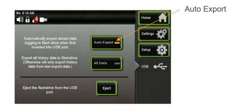
Select the 'Auto Export' feature on the USB menu screen. Insert the flash drive into the chamber's USB port. A new .csv file is automatically created on the flash drive with all the stored history data. The file name nomenclature is "DATE END YYYY-MM-DDTHH-MM\_.csv".
