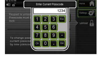
Enter the digits "1 2 3 4"; press (Enter) when complete. The Control Lock Icon will change back to the "unlocked" position.
