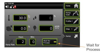
When (Wait for Process) button is selected, the parameter step will wait until the setpoints have been reached before proceeding to the next step .
