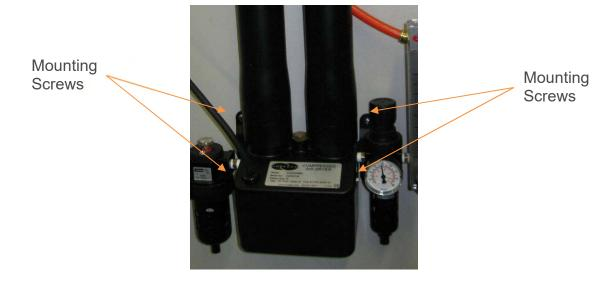
2. Connect dryer package power cord and 3/8" orange tubing into the dryer panel on the chamber
