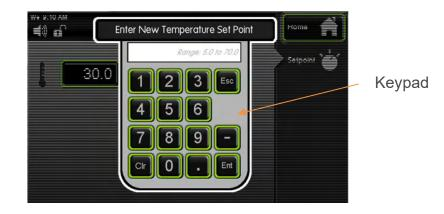
A temperature setpoint window will appear. Enter the temperature setpoint by using the
