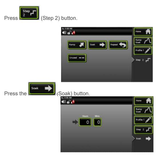
Press (Hours) and or (Mins) button(s) for desired soak time. This feature allows the unit to stay at the Ramp value for a specified amount of time before going to the next Step.
