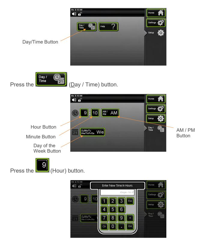
The Enter New Time in Hours window will appear. Enter the hour by using the keypad
