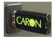
The DLOG301 option provides the customer with a means of logging data electronically for viewing at a later date. Logged variables are Temperature, Humidity,  $CO_2$  and Light Intensity (but only if the chamber is equipped with those features.) All data is time-stamped with year, month, day of the month, hour, minute, 24 hour time (ISO 8601 format). This data is stored internally in the chamber in non-volatile memory.
