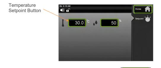
Once the Setpoint screen appears, press the (Temperature Setpoint) button. (In this example the temperature setpoint initially has a value of '30.0'; this will vary with different initial setpoint values.)
