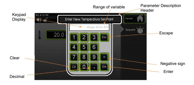
The Parameter Description Header tells what parameter is being changed. The Keypad Display shows allowable values of the parameter being changed (initially) and displays the entered value (when a button is pressed).
