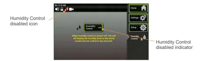
When the humidity control is disabled the toggle button indicator is off and the humidity control icon in the status bar has a red circle around it.
