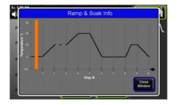
When a ramp cycle has more than 10 steps, there is a button that will allow the steps to continue to the next profile. With the Profile screen open, at the bottom of the screen
