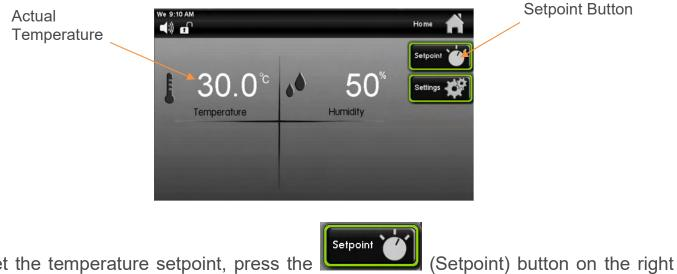
To set the temperature setpoint, press the side of the screen.
