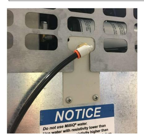
A water inlet fitting on the back of the unit and  $\frac{1}{4}$ " black tubing are provided to connect the water supply to the chamber. Connect an appropriate water supply to the fitting. Incoming line pressure should be regulated to not exceed 80 psi.
