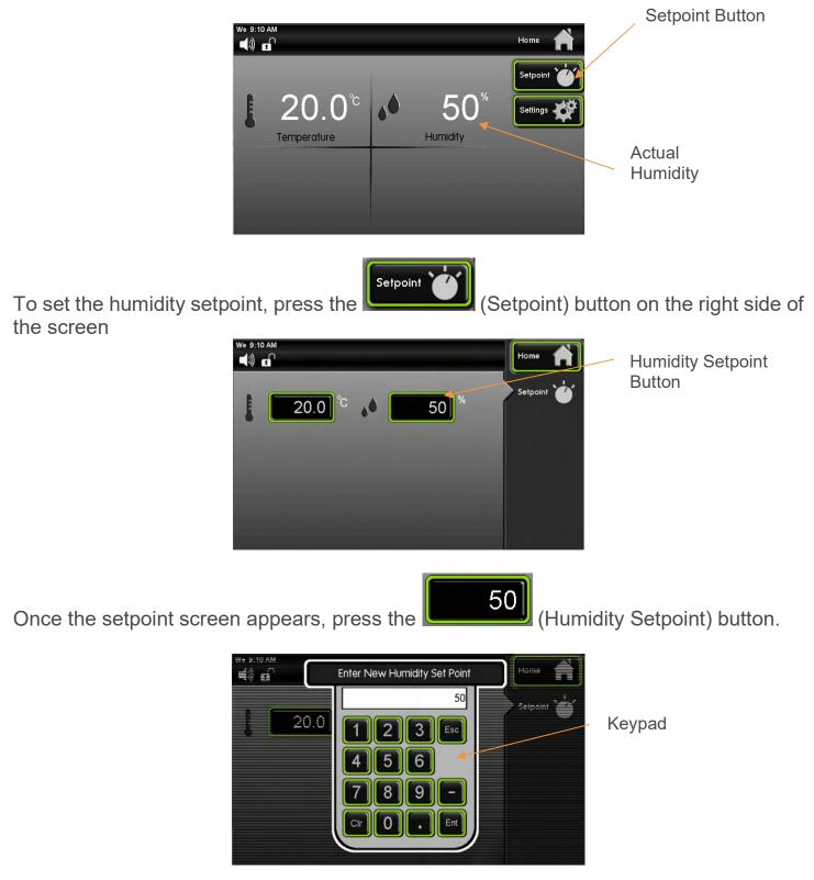
Enter the new humidity setpoint on the keypad as desired and press [Enter] (Enter) when complete.
