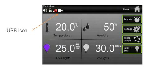
USB icon appears in in Status bar indicating that data is being written to flash drive. To retrieve the data press the 'Eject' button, then insert the flash drive into a computer to upload the data.
