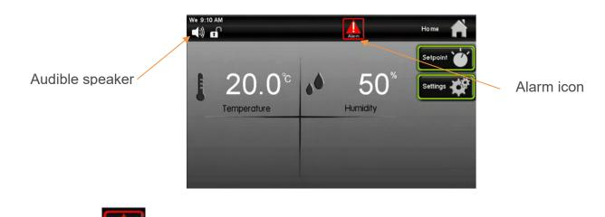
The flashing (Alarm) icon will appear on the status bar.
