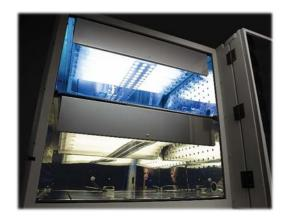
By combining tight uniformity with closely spaced bulbs, the full Q1B-specified exposures can be achieved within 42 hours (35 hours VIS, 7 hours UVA, -2 and -3 models only).
