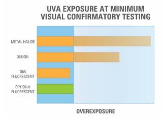
Due to fluorescent D65 lamp's lower UVA irradiance, they overexpose in the visual region. Ideally, illuminance and UVA irradiance would be controlled independently. Selective overexposure can lead to false results, and mistaken and potentially costly product packaging solutions based on that data. This problem is only alleviated by using two different light sources, as specified in Option II.
