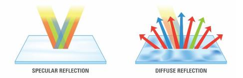
The lamp's spectral power distribution is best preserved by using specular aluminum on interior reflective surfaces. Specular aluminum uniformly reflects light across both UVA and photopic spectrums. It is available with a 95% total reflection (DIN 5036-3) and only 0.01% diffuseness at 15°. Specular aluminum's superior reflective properties outshine mirrored stainless steel and white painted surfaces for not only illuminance reflection but also UVA irradiance.
