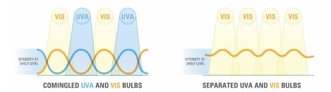
The simplest and most repeatable way, therefore, to avoid varying UV/VIS exposure ratios within a test batch is to divide UV and VIS exposure into separate physical areas, each separately measured and controlled.
